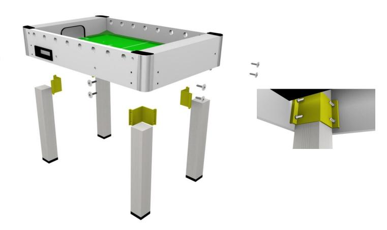
Set the L shaped bracket internally the table boby and insert the aluminium leg inside the L bracket.
